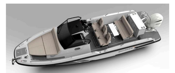
The design consists of three seats at the helm, a comfortable sofa in aft together with a dining table as well as a wet bar with a built in hand basin and storage.
