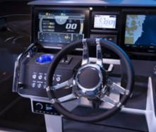
The clean driver-focused helm is designed ergonomically; all panels and switches are centrally positioned around the skipper. The console fits two 12" Garmin plotters. ←
